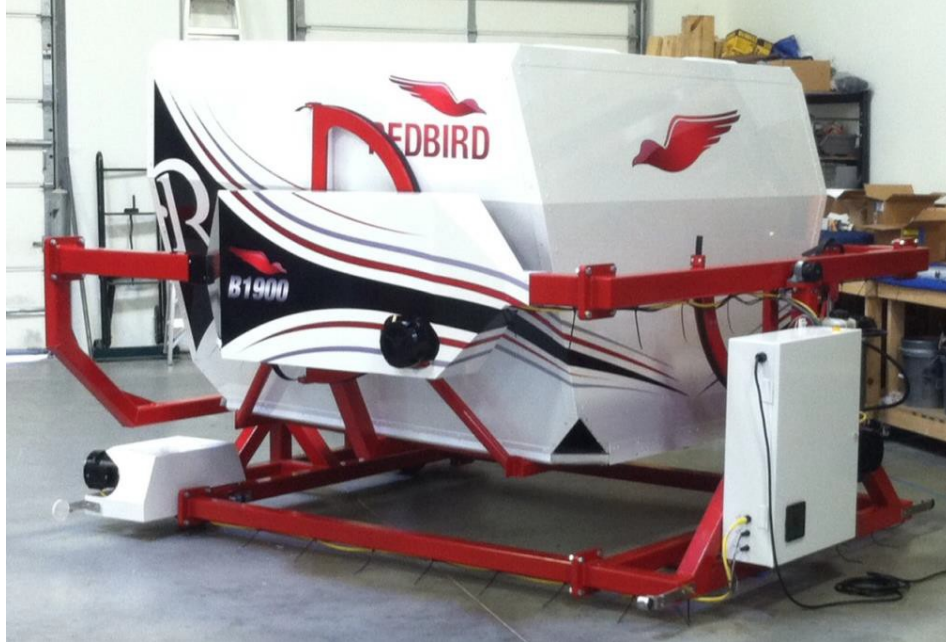
Image 30: Motion Platform and Cockpit Enclosure
