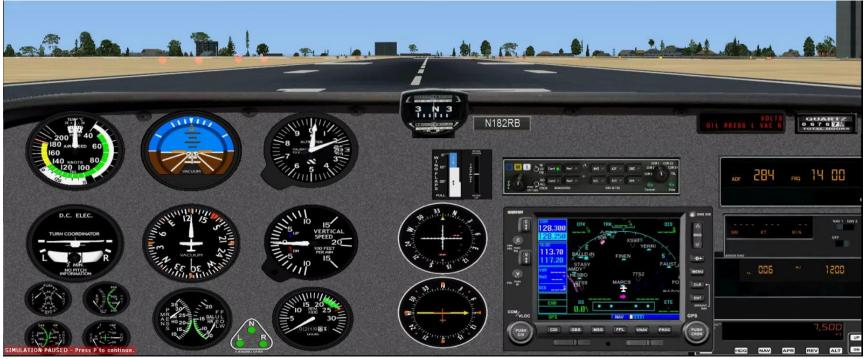
Figure 26: C182 – Analog, CS Prop & Retractable Gears
