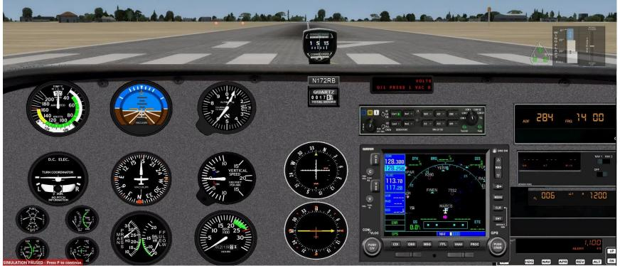
Figure 21: C172 – Analog, CS Prop & Retractable Gears
