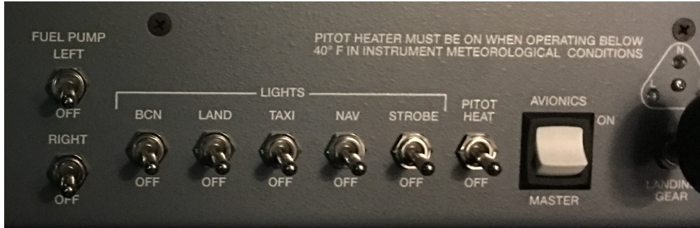
Image 4.1: SwitchPanel (Lower Left)
