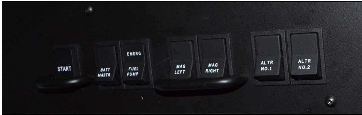
Image 17: Overhead Switch Panel (Pilot)
