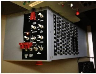
Image 20 Circuit Breaker Panel and Left Switch Panel
