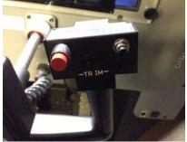
Image 14 Co-Pilot Yoke Switches – Right
