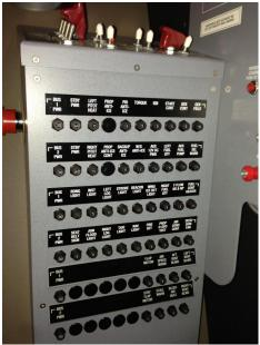
Image 18 Circuit Breaker Panel Pilots Side
