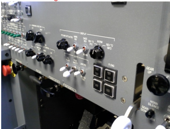
Image 17: Pilot Lower Switch Panel (Right)
