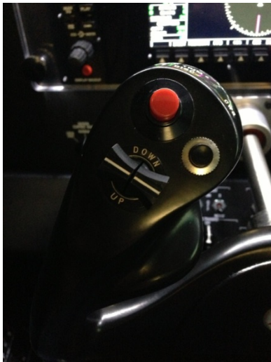
Image 9: Pilot Yoke Switches – Left
