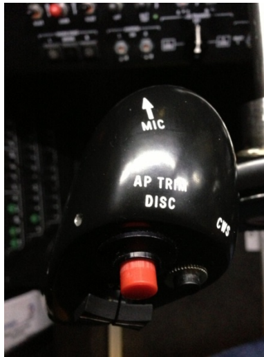
Image 10: Pilot Yoke Switches – Left
