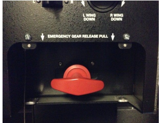
Image :23 Emergency Gear Extension Handle
