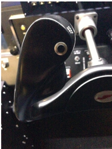
Image 12: Co-Pilot Yoke Switches – Left
