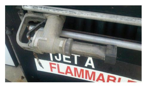
Figure 2-11. A jet fuel filler nozzle is flared at the end to prevent an inadvertent insertion into an AVGAS tank.
