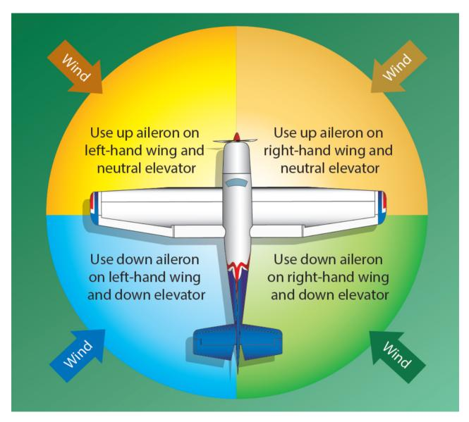
**Figure 2-15.** *Control positions of the nosewheel airplane.*
