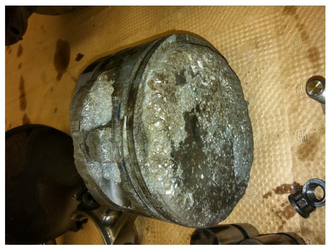
Figure 2-9. An aircraft piston showing damage that occurred in just minutes as a result of detonation and overheating.
