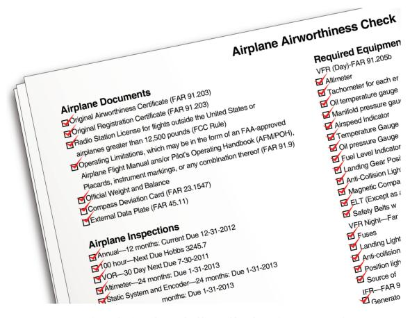
Figure 2-4. A sample airworthiness checklist used by pilots to inspect an aircraft.
